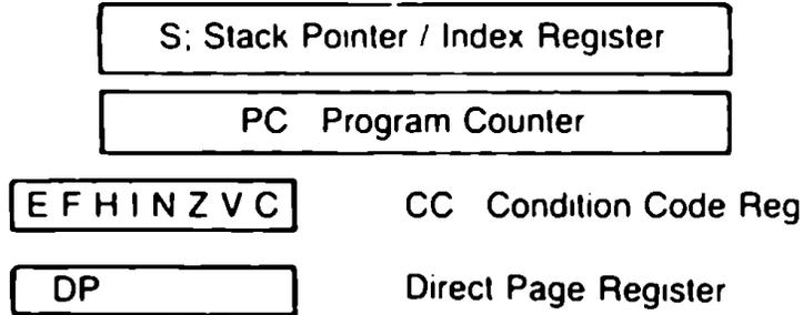
A and B are 8-bit general purpose accumulators used for arithmetic and logical operations. They can also be considered together as the 16-bit D accumulator for certain instructions.
