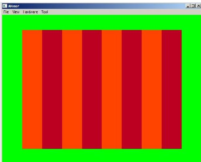
Besides the exact cycle count to hit the correct byte to have the right switching, you can see that we have added 'dummy' cycles to sum a total of 57 cycles so that without any synchronization of interrupts the program will be processing all of the lines ... even the non visible, of course, if this doesn't matter as is the case.
